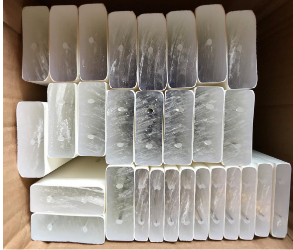
Figure 4. Extruded scintillating bars produced at FNAL with one and two holes for WLS fiber insertion.
