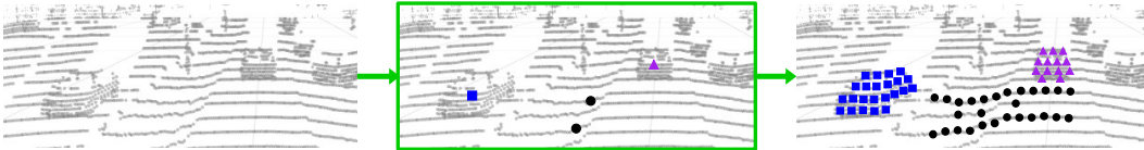
Figure 1: Illustration of the proposed Grounded Point Colorization (GPC) . We pre-train the detector backbone by colorization (left to right), taking the hints on a seed set of points (middle) to overcome the inherent color variation. We show that the middle step is the key to learning the semantic cues of objects from colors.
