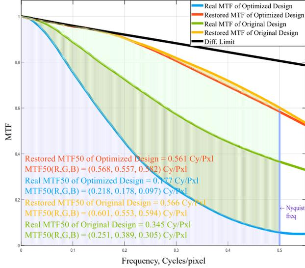
Figure 9: The MTF enhancement of the original and optimized design. All MTF of the lenses mentioned in this article is calculated by *imatest*<sup>®</sup> for reference.
