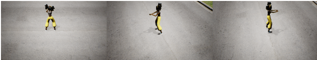
Fig. 6. Airsim simulation in Unreal Engine. We use Airsim simulation to obtain the ground truth of the human actor surface and compare it against our reconstruction results. We use the Computer Vision mode of the Airsim, where the images of the actor are taken in the first-person view of the camera.
