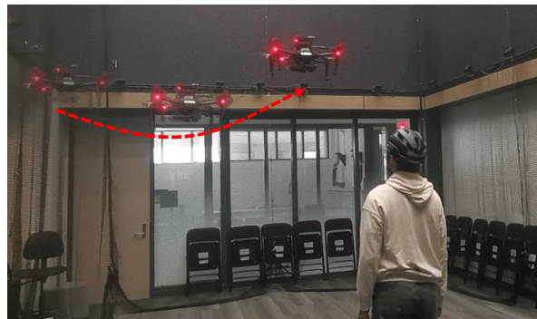
Fig. 1. Capturing images with a flying camera for the high-fidelity reconstruction of a dynamic actor. We build a drone system to capture a dynamic actor’s high-fidelity 3D reconstruction and study the view planning strategy for better reconstruction quality.
