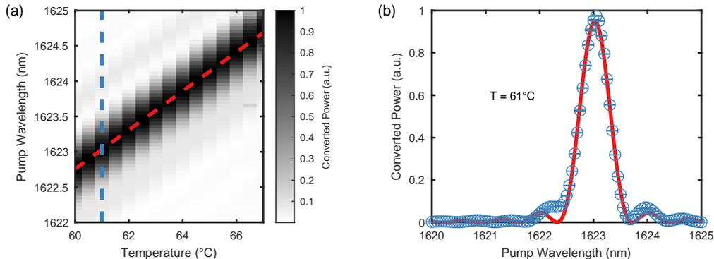
FIG. S3. **PPLN transfer function** **a)**, Normalized conversion efficiency as a function of chip temperature  $T$  and pump wavelength, showing tunability of the phase-matching condition by  $0.28 \text{ nm}/^\circ\text{C}$  (red dashed line). **b)** A cross-section of the transfer function at  $T = 61^\circ\text{C}$  (blue dashed line in **a**). Fitting the expected sinc function to the data (data in blue, fit in red) shows a phase-matching bandwidth of around  $0.8 \text{ nm}$ .
