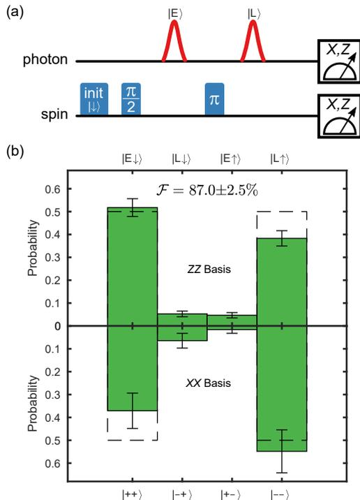
FIG. 5. (a) Pulse sequence for generating and verifying photonic state transfer. (b) Fidelity of the photon-to-spin mapping. Measurement of a transmitted photon in the  $X$ -basis heralds state transfer, whereupon the spin is read out in the  $X$ - or  $Z$ -basis, as appropriate for the photon state sent.
