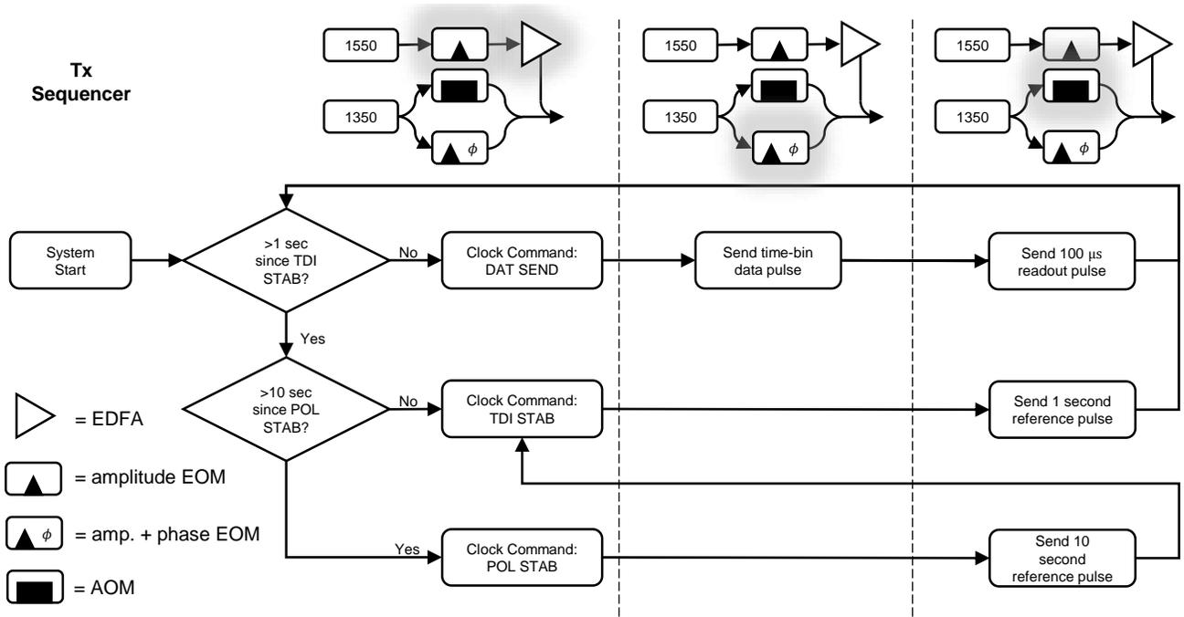
FIG. S5. **Transmitter experimental sequence.** Logical flowchart for the AWG sequencer used to control Alice's transmitter. Inset diagrams show a simplified version of the transmitter hardware, with glows indicating components which are being actively controlled during given portions of the sequence.
