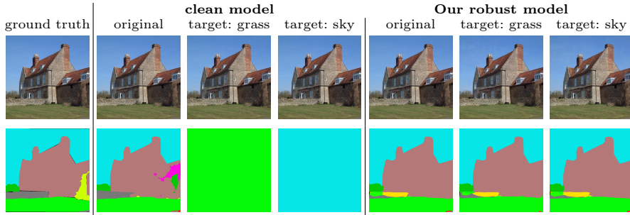
Fig. 1: Effect of adversarial attacks on semantic segmentation models. For a validation image of ADE20K (first column, with ground truth mask), we show the image perturbed by targeted \ell_\infty -attacks ( \epsilon_\infty = 2/255 , target class “grass” or “sky”), and the predicted segmentation. For a clean model the attack completely alters the segmentation map, while our robust model (UPerNet + ConvNeXt-T trained with 5-step PIR-AT for 128 epochs) is minimally affected. For illustration, we use targeted attacks, and not untargeted ones as in the rest of the paper. More illustrations in Appendix D.
