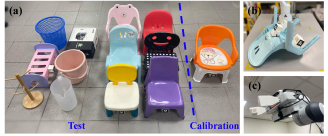
Fig. 4. Experiment Details. (a) Robot Experiment Data. The right chair is used for calibrating the perception, imagination, planning, and control. The rest 12 objects are previously unseen and are used for testing our method and robot system. (b) A test chair with handles attached under the seat. (c) The gripper is mounted with two RGB-D cameras for scanning and tracking respectively.
