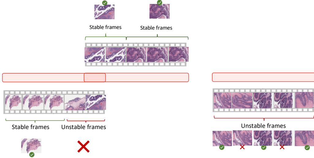
Figure 7: Representative Frame Identification. If a Stable frame is found by Algorithm 1 within the candidate regions, we use it as the representative frame. If not, we use the most dissimilar frames among unstable frames.
