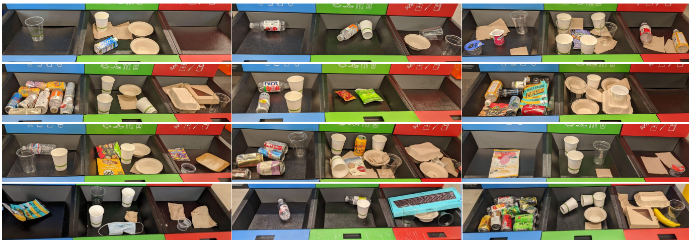
Fig. 4: Waste scenarios used for evaluations. Top 3 rows show the 9 in-distribution scenarios. The bottom row shows the held-out-scenes, containing objects previously seen neither in the real world nor in simulation, such as the keyboard, banana and face-mask.
