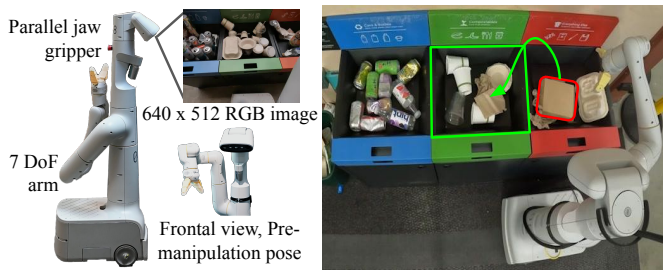
Fig. 2: The experimental platform. left : Our mobile manipulator with a 7 degree-of-freedom (DoF) arm and a parallel jaw gripper. right : The sorting task demonstrated by an example: A compostable food container (red box) is misplaced in the landfill tray. Once the robot arrives at its initial state in front of the waste station with the arm above the station, it executes a trained or scripted policy that identifies misplaced objects and moves them to the correct bin. In the case of this example, the robot would receive a reward for moving the food container into the compost tray (green box).
