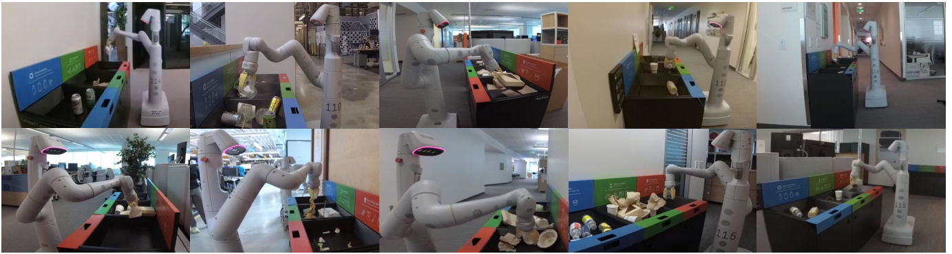
Fig. 6: Example scenes from the deployment sites in 3 different buildings, showing the robot interacting with waste stations used by people over the course of their standard daily routines. Note the high variability in quantity and contamination levels.
