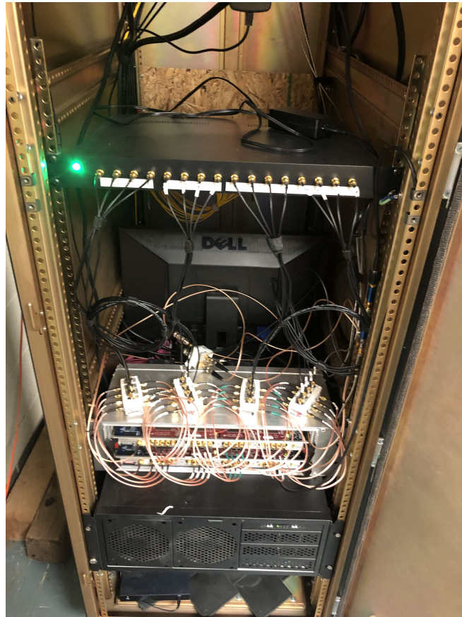
Figure 8: A picture of the digital backend inside the electromagnetically-compliant rack. From the top: The RFoF receiver, the ICE boards, and the Recorder node. The base of the rack holds power supplies for the ICE boards and a gigabit switch for the internal network.
