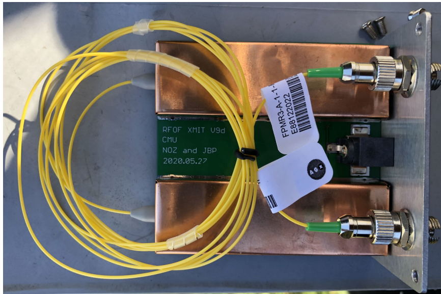
Figure 6: The RFoF transmitter, as seen inside its electromagnetically compliant enclosure.
