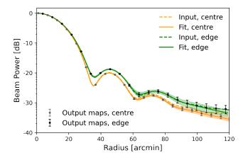
Figure 10. Best-fit beam profiles generated from 3 months of Jupiter simulations for the 93 GHz frequency band, performed with an input beam model for a centre (orange curve) and an edge pixel (green curve). The input beams (orange/green dashed lines) and data points (gray/black errorbars) of the fitted models are also shown.
