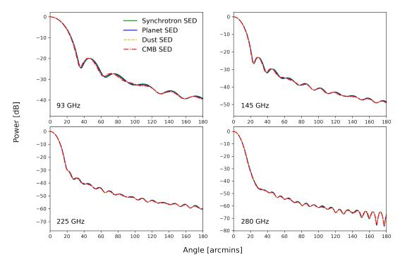
**Figure 19.** Beam profiles for four models constructed using Equations A1 and A2 where the frequency scaling matches the SED of CMB (red curve), planets (blue curve), galactic dust (orange curve) and synchrotron emission (green curve). The plots refer to four frequency bands centred on 93, 145, 225, and 280 GHz and include the case where no frequency scaling was implemented (black dashed line), for reference.
