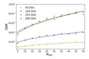
Figure 14. Signal-to-Noise ratio as a function of the number of simulated ~ hour-long Jupiter observations for four frequency bands centred on 93, 145, 225 and 280 GHz. The circles represent SNR values estimated by determining the noise levels of the maps, and the dashed lines represent the best fits of the data points to a  $A\sqrt{N_{obs}} + B$  model.
