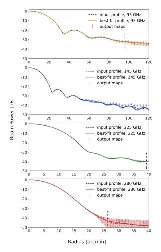
Figure 15. Best-fit beam profiles for the boresight pixel beam model at the 93-, 145-, 225- and 280-GHz frequency bands. Note that the panels showing the 93- and 145-GHz results have different horizontal range than those showing results for 225- and 280-GHz. The vertical black line represents the transition between the core and wing fit.
