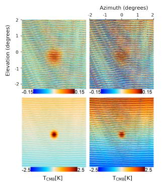
Figure 12. Binned data of a single,  $\sim$  1-hour, Jupiter observation for all detectors in the centre wafer at 93 (top) and 280 GHz (bottom) that have the mean temperature subtracted and have no correlated noise modes removed. The left and right panels represent simulations that include atmospheric emission of PWV = 0.5 and 2.5 mm, respectively.
