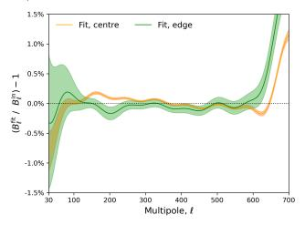
Figure 11. The beam transfer function bias, as compared to the input model, generated from 3 months of Jupiter simulations for the 93 GHz frequency band, performed with an input beam model for a centre (orange curve) and an edge pixel (green curve). The band around the solid lines represents the  $1\sigma$  error envelope determined from the beam error modes.
