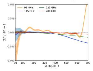
Figure 16. Beam transfer function error with respect to the input beam per frequency band for the beam models of Figure 15.
