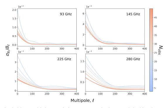
Figure 21. Standard deviation of the beam transfer function uncertainty distribution, as calculated from the 10 strongest error modes, divided by the best-fit transfer function value. The standard deviation is plotted versus the number of input observations provided to beamlib, for four frequency bands centred on 93, 145, 225 and 280 GHz.
