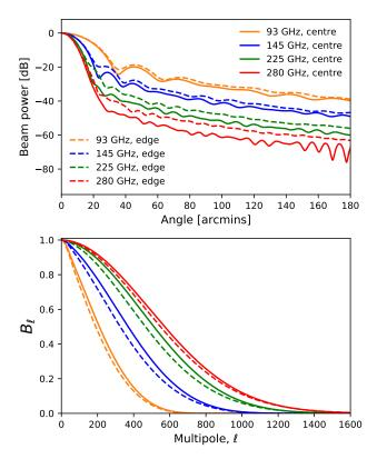
Figure 2. Top: Beam profiles of the band-averaged input beam models for the four SO SATs frequency bands discussed in this paper. Solid and dashed lines show the cases for a detector placed on the center (0 cm) and the edge (18 cm) of the focal plane, respectively. The beam profiles are computed by radially binning the 2D band-averaged beam maps. Bottom: Transfer functions for the beam models whose profiles are presented in the top plot.
