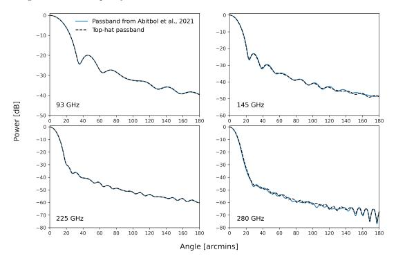
Figure 18. Logarithmic profiles of beam models where a top-hat (black dashed line) and a more realistic (blue line) passband was assumed. The realistic passband was taken from Abitbol et al. (2021), and the results refer to four frequency bands centred on 93, 145, 225, and 280 GHz.
