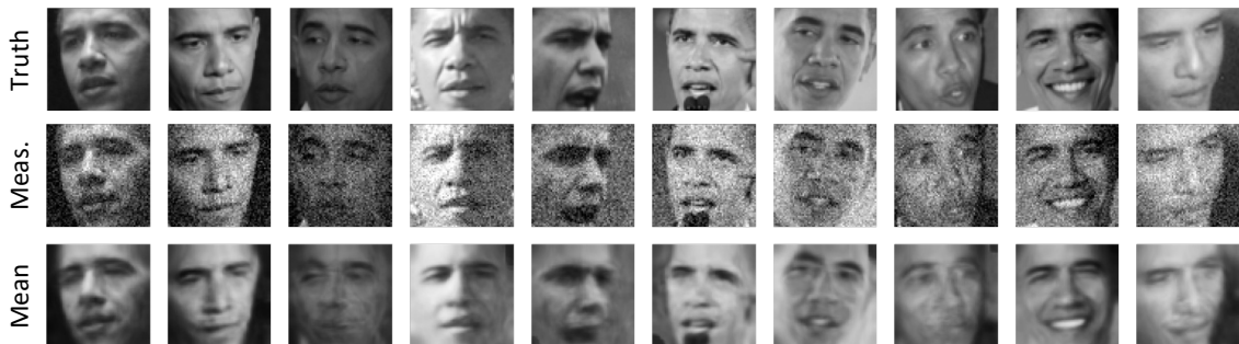
Fig. 16: Denoising 95 images of celebrity B. We demonstrate our method described in Section III-B of the main body using 95 noisy images of a celebrity. These results are of celebrity B, but correspond to Fig. 5 in the main body. Here we show the ground-truth (top), noisy measurements (middle), and mean reconstruction (bottom) for a subset of the 95 different noisy images. Our reconstructions are much less noisy, recovering sharper features that are hard to discern in the noisy images. Note that no predefined prior/regularizer was used in denoising.
