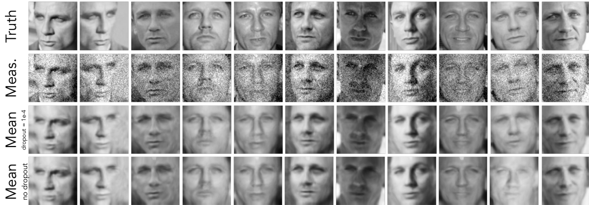
Fig. 15: Dropout ablation with denoising 95 images of celebrity A. We demonstrate our method described in Section III-B of the main body using 95 noisy images of a celebrity. Here we show the ground-truth (row 1), noisy measurements (row 2), mean reconstruction with dropout (row 3), and mean reconstruction without dropout (row 4) for a subset of the 95 different noisy images. The reconstructions with and without dropout have similar image quality. The mean PSNR for with dropout is 27.0 and for without dropout is 27.2.
