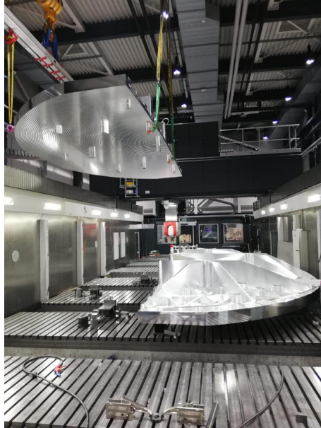
Fig. 3. The two separate reflector halves after rough machining and before they were bolted together. The surface of the reflector is pointed downwards and you can see large aluminum pillars on the surface of the reflector that still need to be removed.
