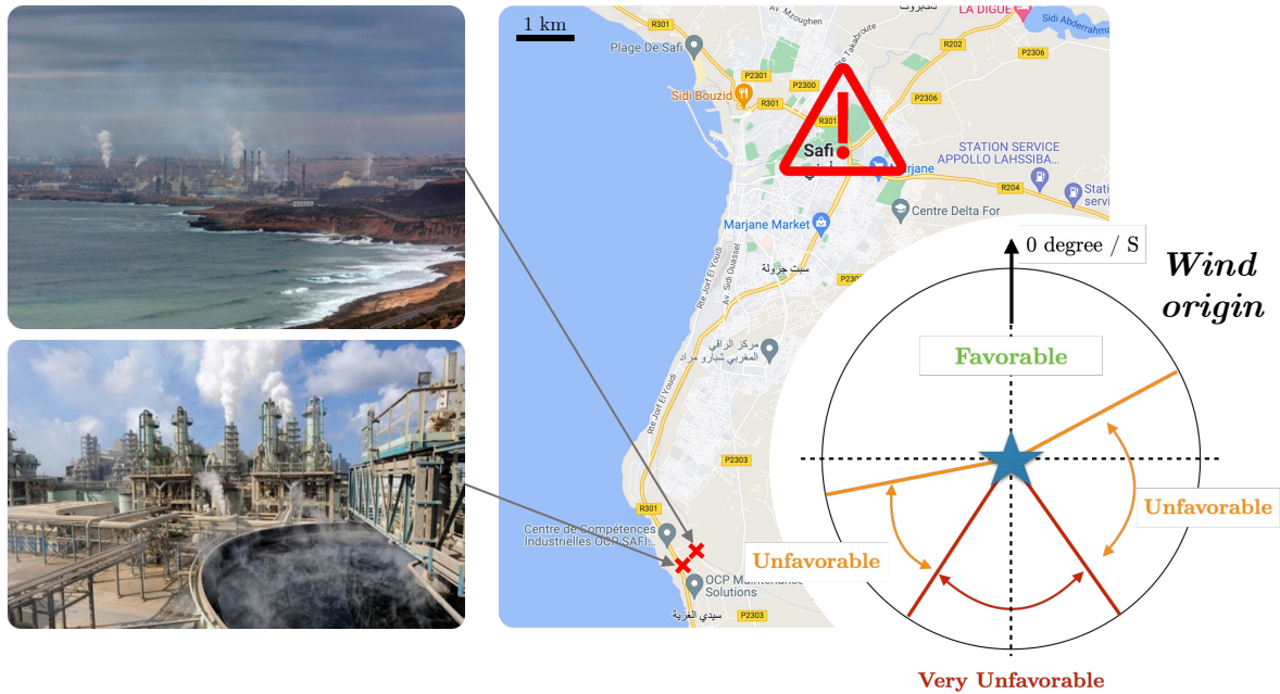
Figure 2: Wind direction and wind speed determine the dissemination of pollutants. Winds coming from the South with low speeds are the most dangerous conditions.
