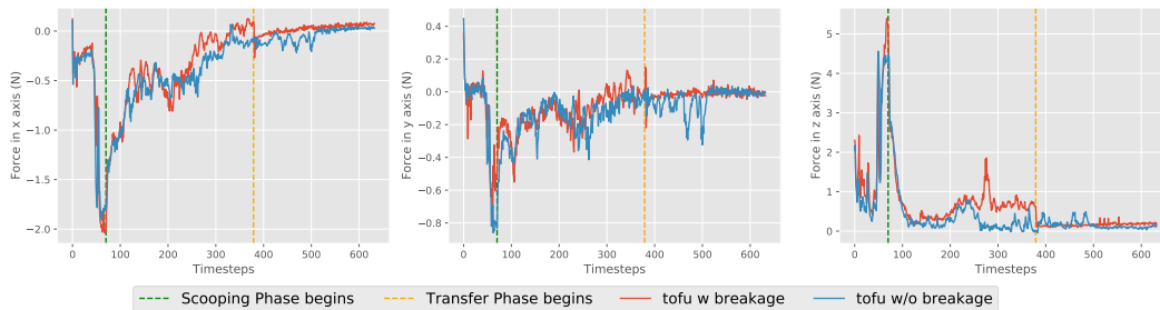
Figure 11: Sensored forces from tofu rollouts: We report the sensed force in the pusher along the x, y and z axes in three phases (Pushing, Scooping, Transfer) for tofu rollouts. The breakage happens around the timestep of the green line where the transition from pushing to scooping starts. We cannot identify the breakage failures purely from the force torque sensing.
