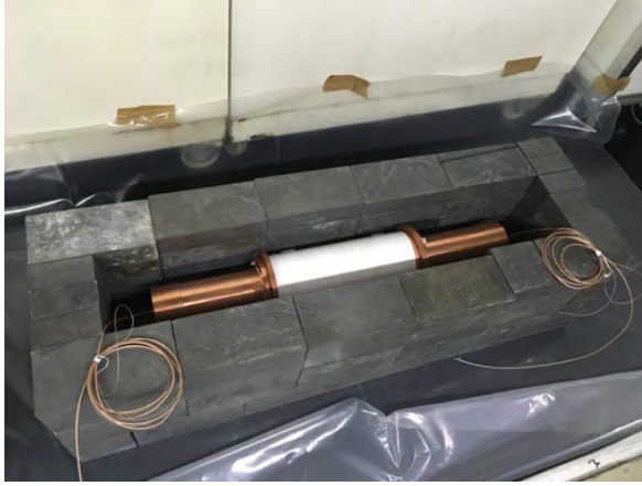
Figure 4: Setting-up the ANAIS blank module in the ANAIS hut, inside a specific lead shielding, 10 cm thick, next to ANAIS-112.
