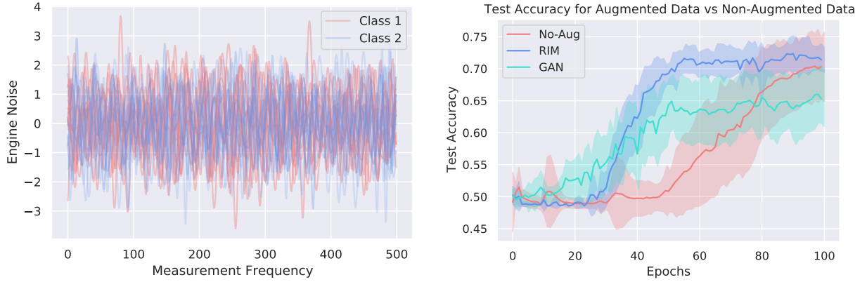
Figure 5: Time series from two classes and Test Accuracy for the Ford Engine Classification with a Convolutional Neural Network with kernel size=3, filter=32, batch size=16, using BatchNorm and Adam optimizer. The test accuracy plot indicates the resulting mean \pm standard deviation from 10 runs.
