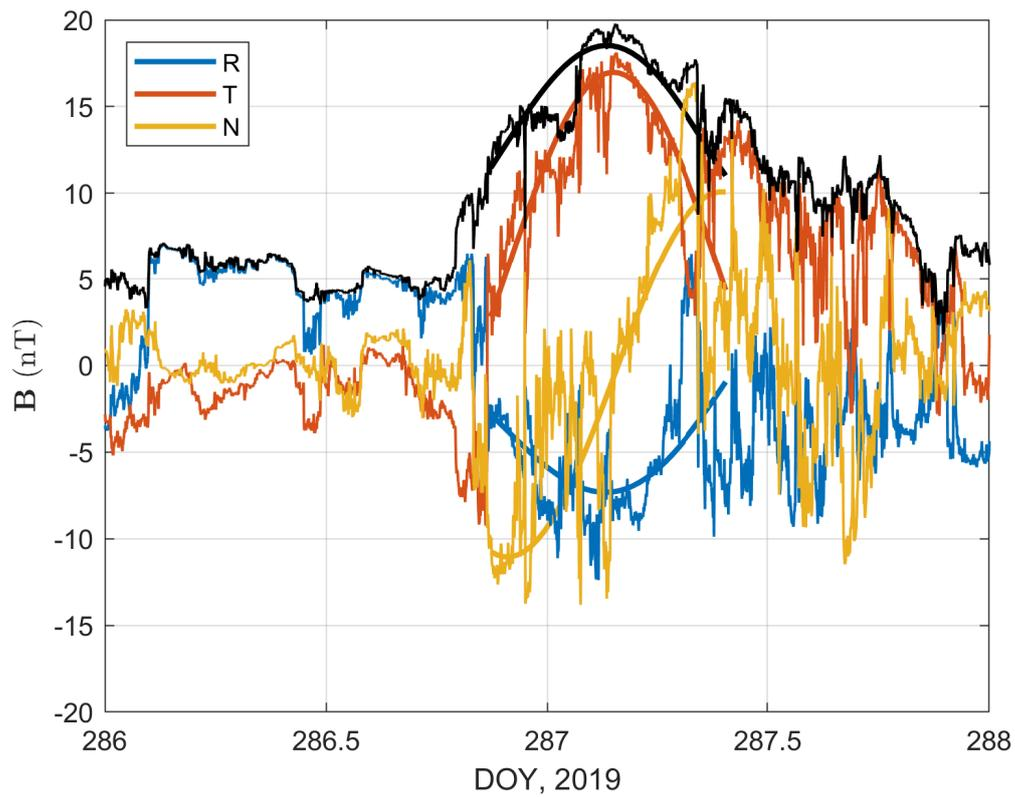
**Figure 3.** The corresponding magnetic field measurements including the magnitude (black) from PSP in the RTN coordinates during day of year, DOY 286 (October 13), and DOY 288, 2019. The smooth curves are the FS model output from the two-spacecraft optimization presented in Section 3.
