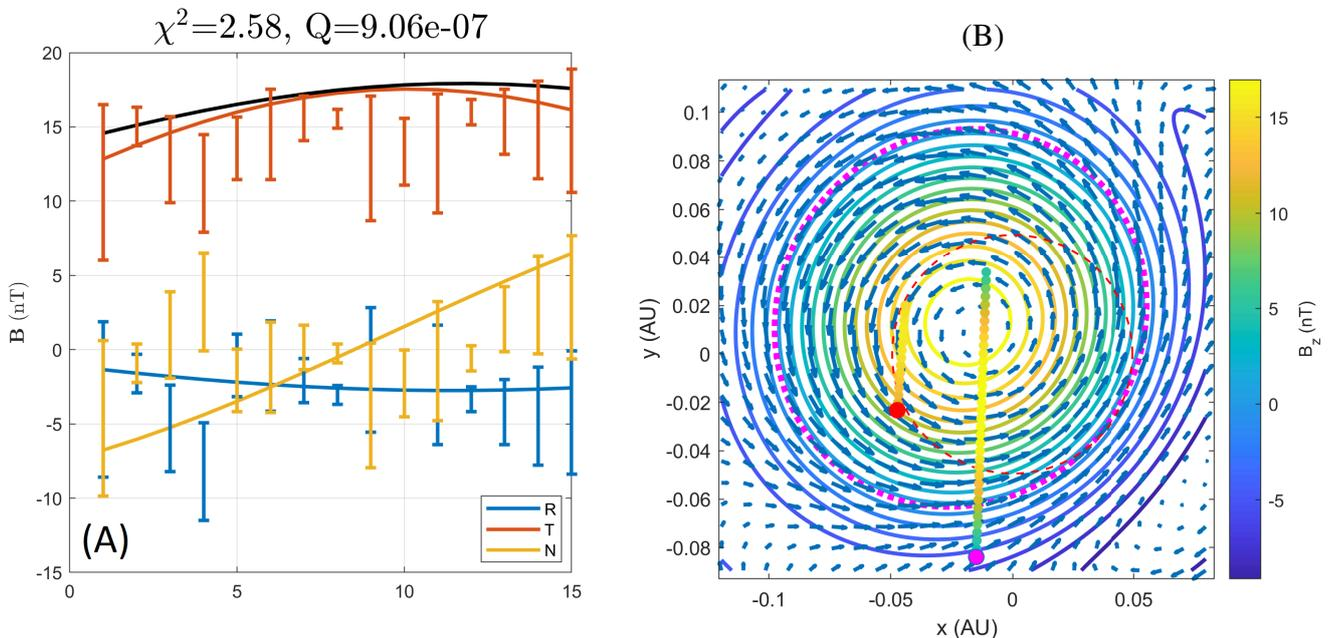
**Figure 8.** (A) The two-spacecraft (STA-PSP) optimization result of the magnetic field components and magnitude (black curve) for the STA data interval. Format is the same as Figure 4. (B) One cross section for the optimal FS model result based on the two-spacecraft (STA-PSP) optimization (with  $a = 0.049$  AU). Format is the same as Figure 5.
