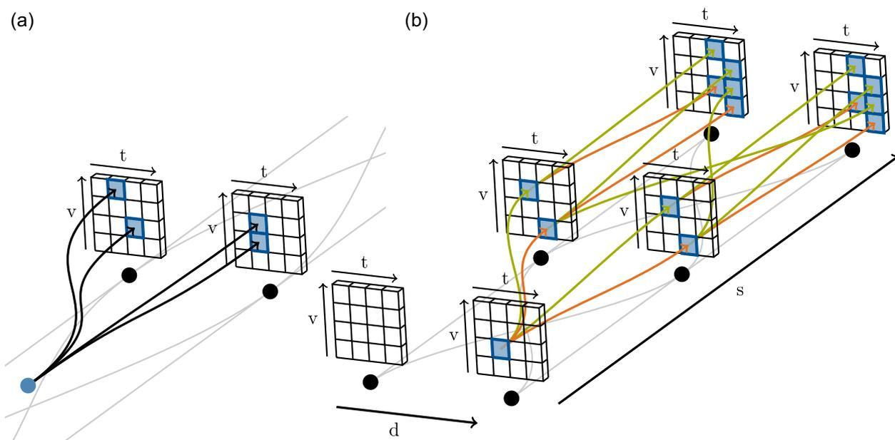
**FIGURE 7** Overview of the short-term and long-term planning steps for the local trajectory planning. (a) Short-term planning step (STPS) and (b) long-term planning step (LTPS). [Color figure can be viewed at [wileyonlinelibrary.com](http://wileyonlinelibrary.com)]
