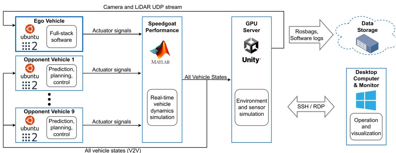
**FIGURE 11** Overview of the TUM HiL architecture. GPU, graphics processing unit; HiL, Hardware-in-the-Loop; LiDAR, Light Detection and Ranging; RDP, remote desktop protocol; SSH, secure shell; TUM, Technical University of Munich; UDP, user datagram protocol. [Color figure can be viewed at [wileyonlinelibrary.com](http://wileyonlinelibrary.com)]
