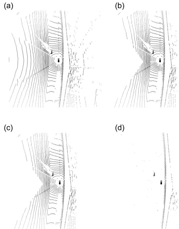
**FIGURE 5** Visualization of the three LiDAR preprocessing steps on an exemplary point cloud. (a) Raw input 74,302 points, (b) after conditional removal 66,585 points, (c) after voxel downsampling 29,502 points, and (d) after ground filter 11,995 points. LiDAR, Light Detection and Ranging.
