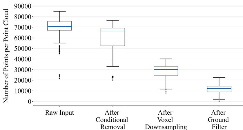
**FIGURE 4** Breakdown of the point reduction for each LiDAR preprocessing algorithm, based on 32,568 point clouds captured during the final run of the Autonomous Challenge at CES on January 7, 2022. LiDAR, Light Detection and Ranging. [Color figure can be viewed at [wileyonlinelibrary.com](https://onlinelibrary.wiley.com/doi/10.1002/rob.22153)]
