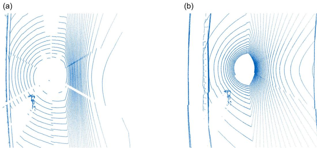
**FIGURE 12** Comparison of real and synthetic point cloud. (a) Real point cloud from the AV-21 and (b) synthetic point cloud from the TUM HiL. HiL, Hardware-in-the-Loop; TUM, Technical University of Munich. [Color figure can be viewed at [wileyonlinelibrary.com](https://onlinelibrary.wiley.com/doi/10.1002/prob.22153)]
