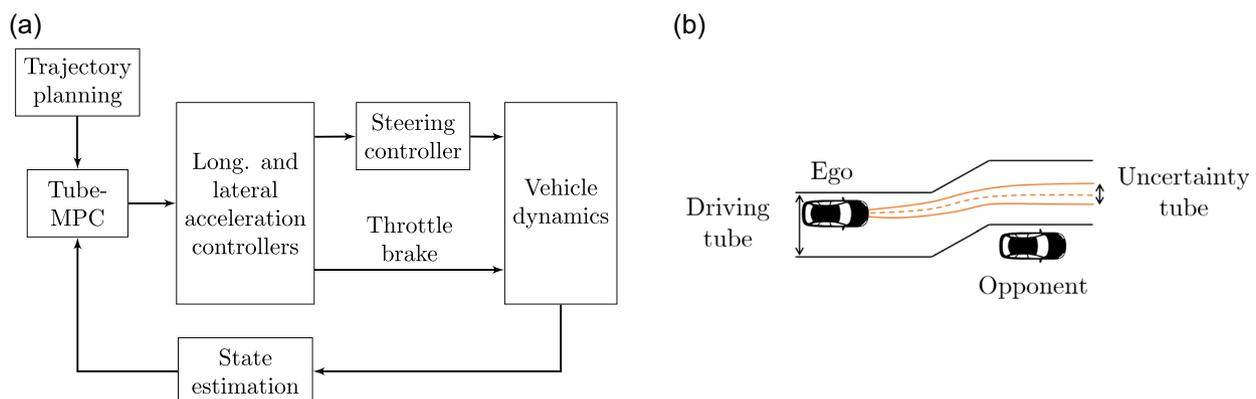
**FIGURE 8** Overview of the motion control algorithm based on Tube-MPC. (a) Internal motion control structure and (b) driving and uncertainty tubes. MPC, Model Predictive Control. [Color figure can be viewed at [wileyonlinelibrary.com](https://onlinelibrary.wiley.com/doi/10.1002/rob.22153)]
