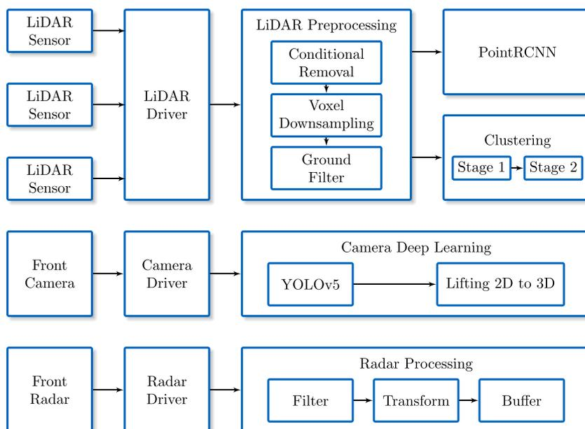
**FIGURE 3** Overview of the object detection pipelines. 2D, two-dimensional; LiDAR, Light Detection and Ranging; RCNN, Regions-based Convolutional Neural Network. [Color figure can be viewed at [wileyonlinelibrary.com](http://wileyonlinelibrary.com)]
