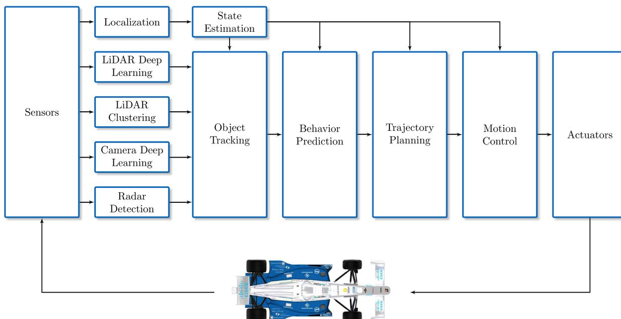
**FIGURE 2** Software architecture of the *TUM Autonomous Motorsport* team. LiDAR, Light Detection and Ranging; TUM, Technical University of Munich. [Color figure can be viewed at [wileyonlinelibrary.com](https://onlinelibrary.wiley.com/doi/10.1002/rob.22153)]
