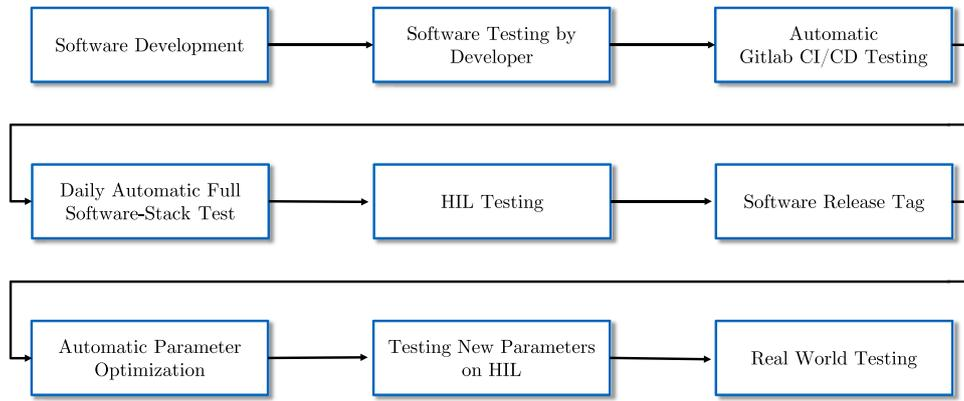
**FIGURE 9** Overall testing workflow. CD, Continuous Development; CI, Continuous Integration; HiL, Hardware-in-the-Loop. [Color figure can be viewed at [wileyonlinelibrary.com](http://wileyonlinelibrary.com)]
