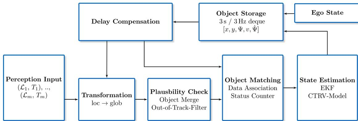
**FIGURE 6** Overview of object fusion and tracking. CTRV, Constant Turn Rate and Velocity; EKF, Extended Kalman Filter. [Color figure can be viewed at [wileyonlinelibrary.com](http://wileyonlinelibrary.com)]
