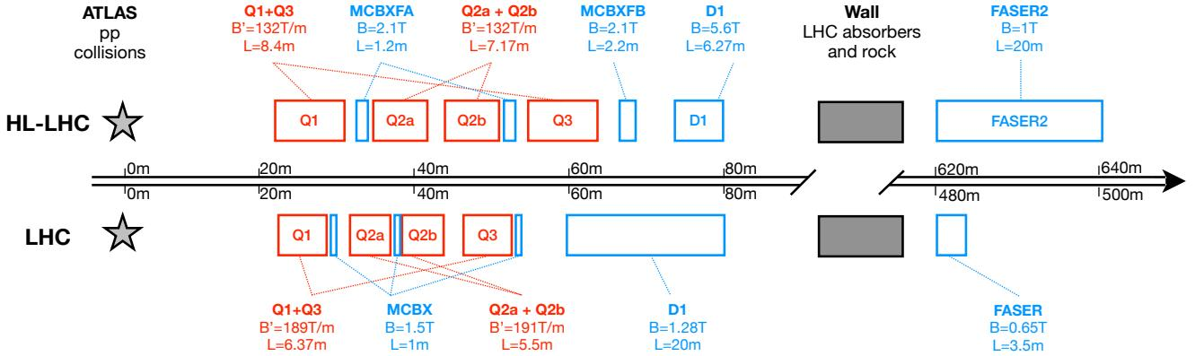
FIG. 1: Considered magnetic fields at the HL-LHC (top) and LHC Run 3 (bottom) downstream from the ATLAS collisions point. We show dipoles in blue and quadrupoles in red, and indicate their corresponding length  $L$ , magnetic field  $B$  and field gradient  $B'$ . Here we have used the magnetic fields as presented in Refs. [44] and [45].
