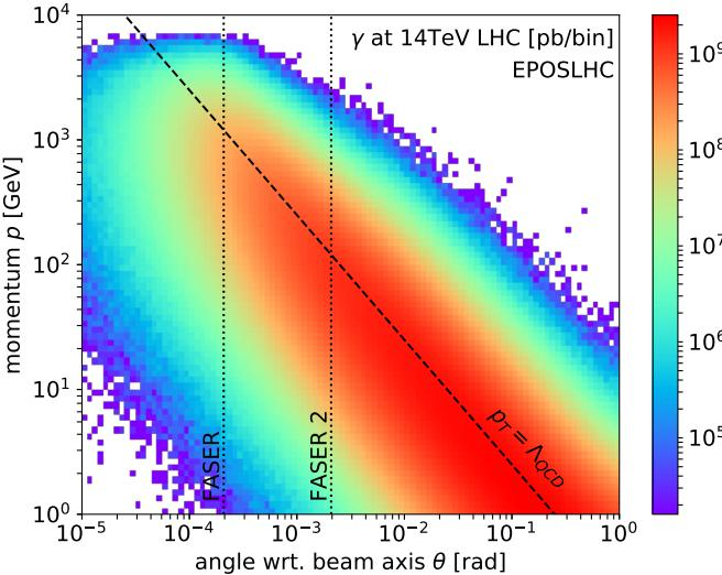
FIG. 2: Differential production rate of photons at 14 TeV LHC predicted by EPOS-LHC in the  $(\theta, p)$  plane, where  $\theta$  and  $p$  are the proton's angle with respect to the beam axis and momentum, respectively. The angular coverage for FASER and FASER 2 are indicated by the vertical dotted lines.
