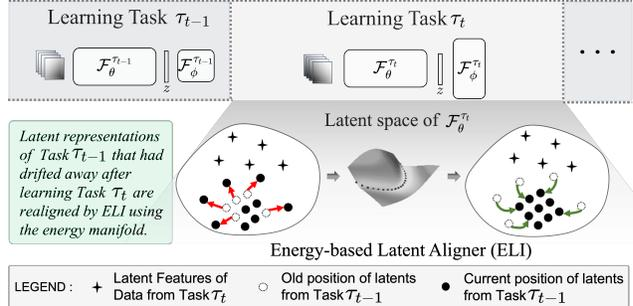
Figure 1. We illustrate an Incremental Learning model trained on a continuum of tasks in the top part of the figure. While learning the current task  $\tau_t$  (zoomed-in), the latent representation of Task  $\tau_{t-1}$  data gets disturbed, as shown by red arrows. ELI learns an energy manifold, and uses it to counteract this inherent representational shift, as illustrated by green arrows, thereby alleviating forgetting.
