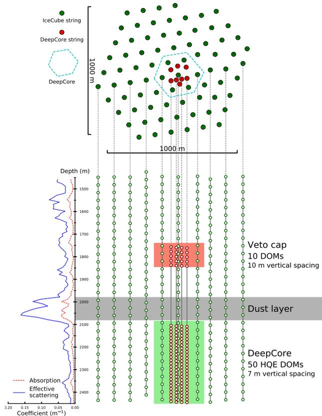
Fig. 1: Schematic view of the IceCube in-ice detector array. The DeepCore sub-array, located at the bottom center, features denser module spacing and allows for the detection of lower energy events compared to the rest of IceCube. Also shown are the depth-dependent effective scattering and absorption coefficients [17]. The zone labeled as “Dust layer” is of inferior optical quality with increased scattering and absorption. The DeepCore array is located below this in the clearest part of the ice.
