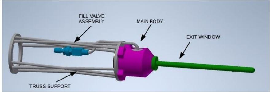
**Figure 1.** The conceptual design of the new gas target cell to be used in E12-12-005 and this experiment.
