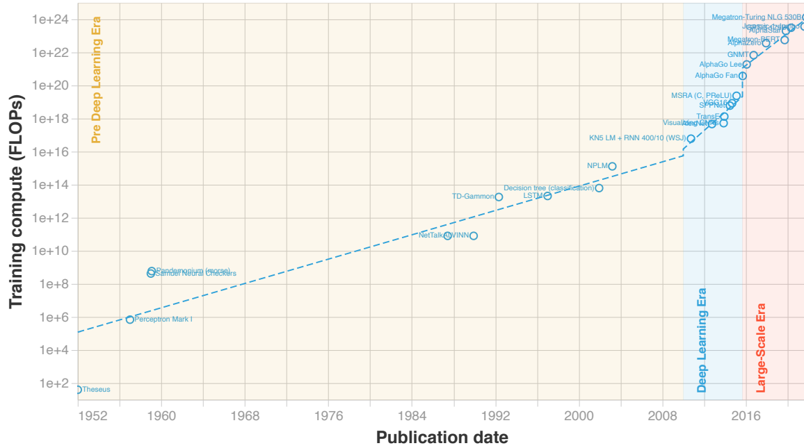
Figure 5: Training compute trend in n = 26 record-setting models between 1952 and 2022. We have excluded AlphaGo Zero and AlphaGo Master from consideration.
