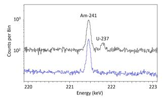
Figure 7: The 221.80-keV peak from <sup>237</sup>U is cleanly separated from the 221.46-keV <sup>241</sup>Am peak. A spectrum from a pure americium source is shown below, which lacks the <sup>237</sup>U peak.
