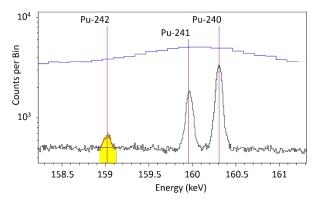
Figure 5: Spectrum detailing the 159-keV region. The peak of interest is highlighted. A typical-quality HPGe spectrum of the same region and same item is shown above the  $\mu$ Cal spectrum.
