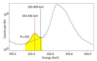
Figure 3: Spectrum from the first run detailing the 103-keV region. The <sup>242</sup>Pu peak of interest is highlighted. Note that this peak appears at a lower energy than reported by Schmorak et al.
