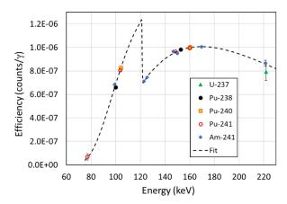
Figure 6: Efficiency calibration curve derived from five radionuclides within the sample. Some points are overlapping. The discontinuity near 120 keV is from the plutonium K-edge.
