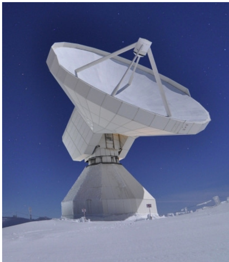
Figure 1. The IRAM 30-m diameter millimeter-wave telescope operating on Pico Veleta in the Sierra Nevada, Spain, at 2900 m altitude.
