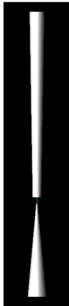
FIG. 5: Model of the best antenna design. Individual 8, evolved in Generation 23. Other individuals are not shown because they are not visually distinguishable from this one.
