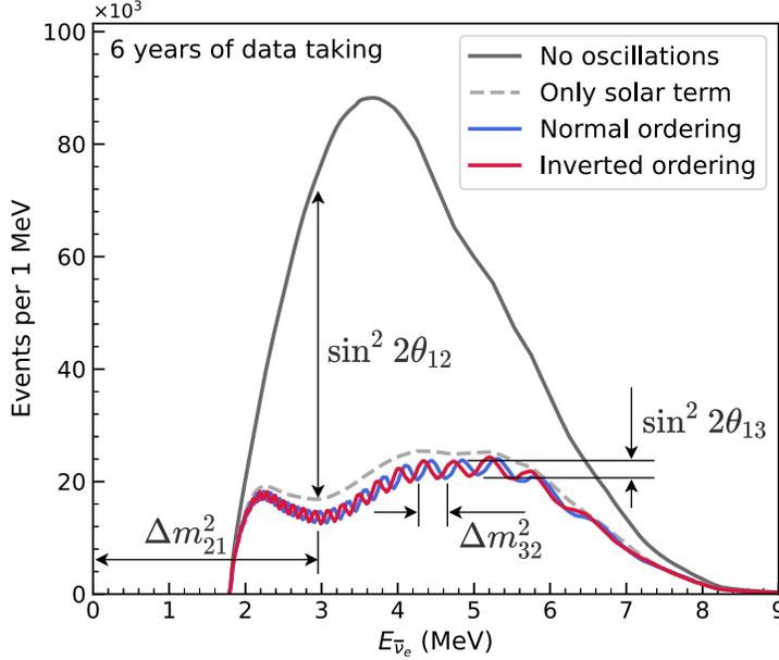
Figure 18: Expected energy spectrum of reactor antineutrinos in JUNO. The black curve shows the un-oscillated spectrum. The dashed curve shows the spectrum assuming  $\theta_{13} = 0$ . The blue and red curves correspond to expected spectra for normal and inverted mass ordering, respectively. The features in the spectrum reflecting the sensitivity in oscillation parameters are demonstrated. Taken from Ref. [273].
