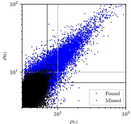
FIG. 4. Distribution of injected SNRs for recovered injections above  $\mathcal{L} = 35$  ( $\sqrt{2\mathcal{L}} = 8.37$ ). Missed injections with network SNR above 12 and detector SNRs greater than 7 (indicated by the shaded contour) are discussed in the appendix.
