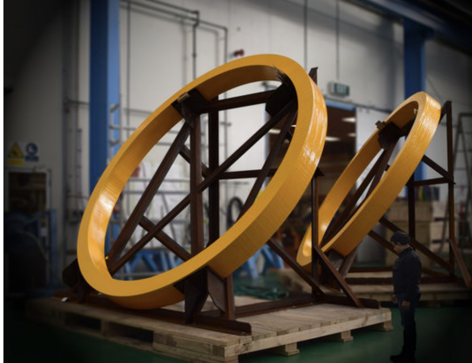
Figure 3.2: Photo of cyclotron coils built by Buckley Systems, Auckland NZ. These coils are 3.33 meters diameter, ours are 4.95. The proportions are about the same as ours. Notice the man in lower right.
