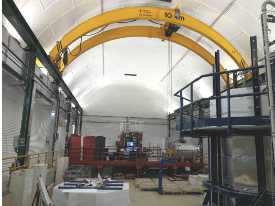
Figure 2.6: Photograph of the interior of the main hall at Canfranc, the underground laboratory in Northern Spain underneath the Pyrenees. The crane, believed to have a 10 ton capacity, elegantly serves the rigging functions in this laboratory. Such cranes would serve well for the rigging needs in the IsoDAR cyclotron and target rooms.
