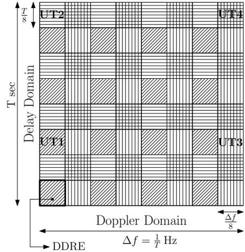
Fig. 1: Allocation of DDREs to the UTs in the IDDMA method ( $M = N = 8, Q = 4, g_1 = g_2 = 2$ ) [21].
