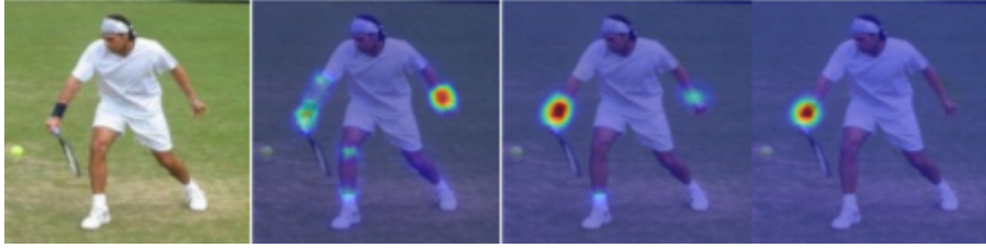
Figure 2.3: This is a sequential architecture across several stages using convolutional networks, spatial context from belief maps, and large receptive fields to create increasingly refined estimates for body part predictions, which in this case is the right elbow [6].
