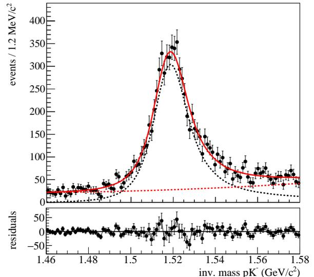
FIG. 4. Example sPlot fit [19] for one bin between  $-(t - t_0) = 0.3 \text{ GeV}^2/c^2 - 0.5 \text{ GeV}^2/c^2$ . Top: The black and red dashed lines show the fit components of signal and background respectively, the red solid line shows the resulting fit to the data (black points). Bottom: Residuals of the total fit to the data.
