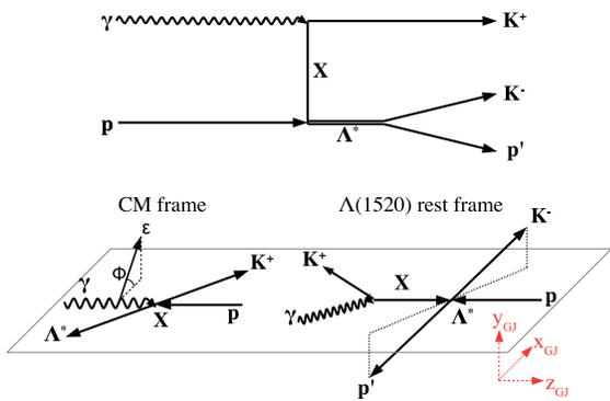
FIG. 1. The Gottfried-Jackson system used in this analysis. The diagram on top visualizes the  $t$ -channel production process expected to dominate at GlueX energies with  $X$  being the exchange particle. The Gottfried-Jackson system is defined in the rest frame of the  $\Lambda(1520)$  (see Eq. (1)). The polarization vector of the incoming beam photon is denoted by  $\epsilon$ .
