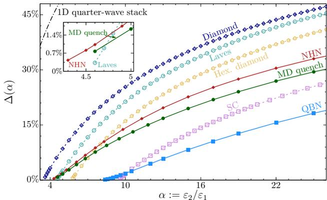
FIG. 2. The *gap plot* shows the optimal gap-to-midgap ratio  $\Delta(\alpha)$  as a function of the dielectric contrast  $\alpha$ . The plot compares three-dimensional photonic crystals (open symbols) to three-dimensional disordered networks (solid symbols). The dashed-dotted line shows  $\Delta_{\text{QWS}}(\alpha)$  for the one-dimensional quarter-wave stack. The inset zooms in on small values of  $\alpha$  where the PBGs first open up for the NHN, MD quench, and Laves networks.
