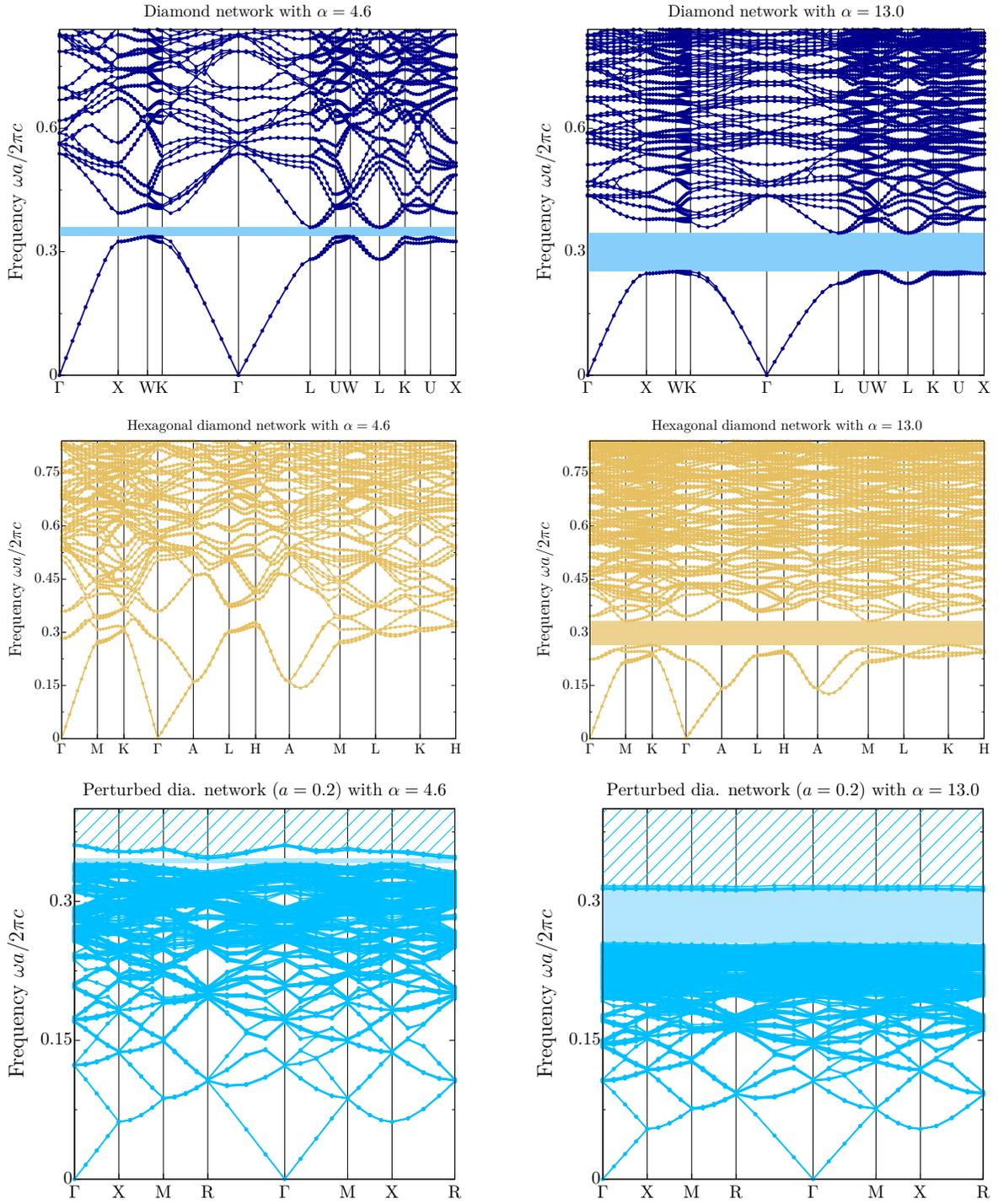
FIG. S1. Photonic band structures for some of the (anisotropic) crystal and perturbed crystal networks at different dielectric contrasts  $\alpha$ ; see also video S2.
