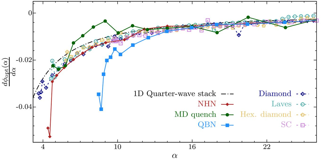
FIG. S3. The derivative of the optimal volume fraction,  $d\phi_{\text{opt}}(\alpha)/d\alpha$  for our crystal and disordered networks approximately agrees at large  $\alpha$  with the analytic result for the 1D quarter-wave stack,  $d\phi_{\text{QWS}}(\alpha)/d\alpha = -1/(2\alpha^{3/2} + 4\alpha + 2\sqrt{\alpha})$ , shown by the dashed-dotted line.
