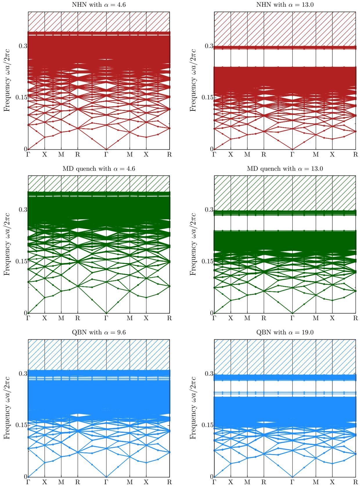
FIG. S1. (Continued) Photonic band structures of (isotropic) disordered networks at different dielectric contrasts  $\alpha$ ; see also video S2.
