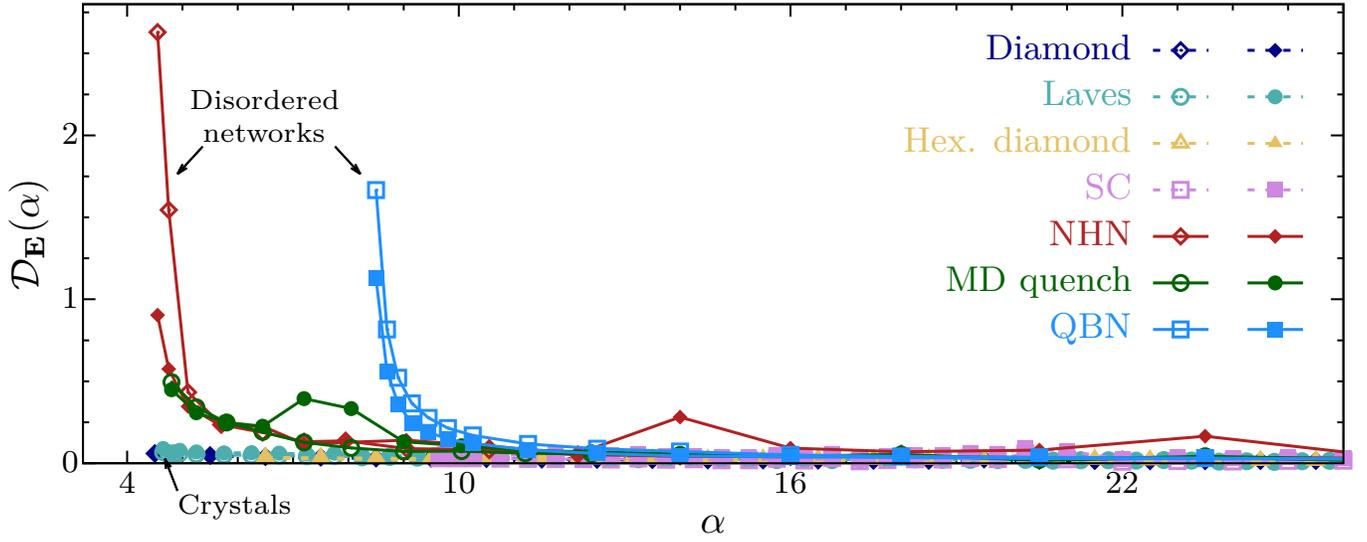
FIG. S2. The average change of the electric field intensity with the dielectric contrast  $\alpha$  for the bands below (open symbols) and above (solid symbols) the PBG. At low  $\alpha$ , the configuration of the electric field changes more strongly for the disordered networks than for the photonic crystals.
