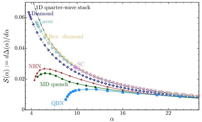
FIG. 3. The *gap-sensitivity plot* shows the slope  $S(\alpha) := d\Delta(\alpha)/d\alpha$  for each of the curves in Fig. 2. For our three-dimensional crystal networks,  $S(\alpha)$  is well approximated by  $S_{\text{QWS}}(\alpha)$  for all  $\alpha$ . For our disordered networks,  $S(\alpha)$  has a maximum at low  $\alpha = \mathcal{O}(1)$  and only converges (approximately) to  $S_{\text{QWS}}(\alpha)$  at larger  $\alpha \gg 1$ .
