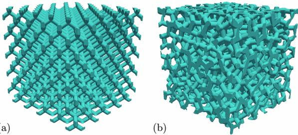
FIG. 1. Photonic networks: (a) the crystal diamond network, where cylindrical rods connect nearest neighbors of a diamond lattice, and (b) the disordered nearly hyperuniform network (NHN) model; see also video S1.
