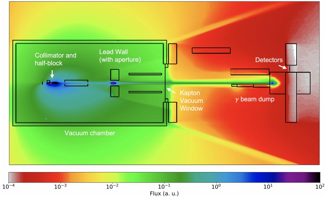
**Figure 10.** Combined photon and charged particle background noise flux throughout the setup. Simulated in Geant4. Lead walls shield the SPD location from direct sight lines to heavy noise sources such as the  $\gamma$  collimator and first lead wall aperture (labelled for clarity).
