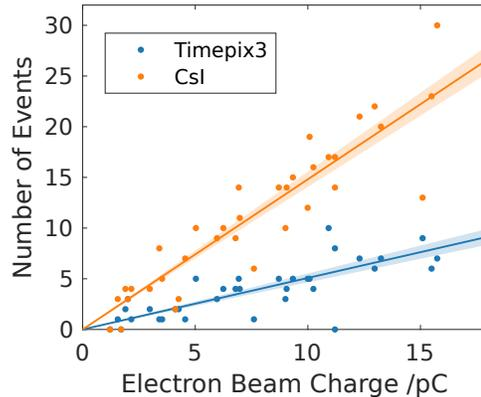
**Figure 11.** Variation of number of background events measured with electron beam charge on the Timepix3 and CsI detectors. Orange: CsI detector, Blue: Timepix3 detector. Shaded regions represent  $1\sigma$  confidence interval on the linear fit.
