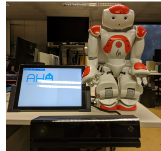
Fig. 5: System prototype that includes a Kinect sensor to track a patient’s exercise and a social robot, NAO and a visualization interface to provide gesture-based, audio, and visual feedback on patient’s performance
