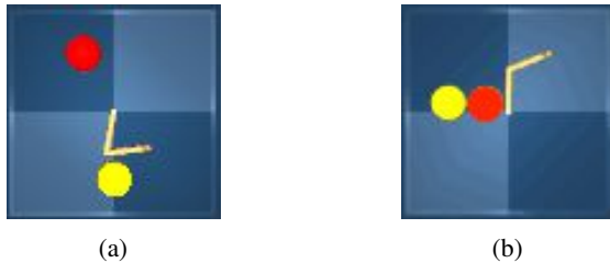
Figure 8. Reacher environment during demonstration time (a) and policy training time (b). During demonstrations, the uncertain region (red) is far from the robot arm and the goal (yellow), but during policy optimization the goal position is randomized and sometimes the uncertain cost region is in the way forcing the agent to either go around or through it.
