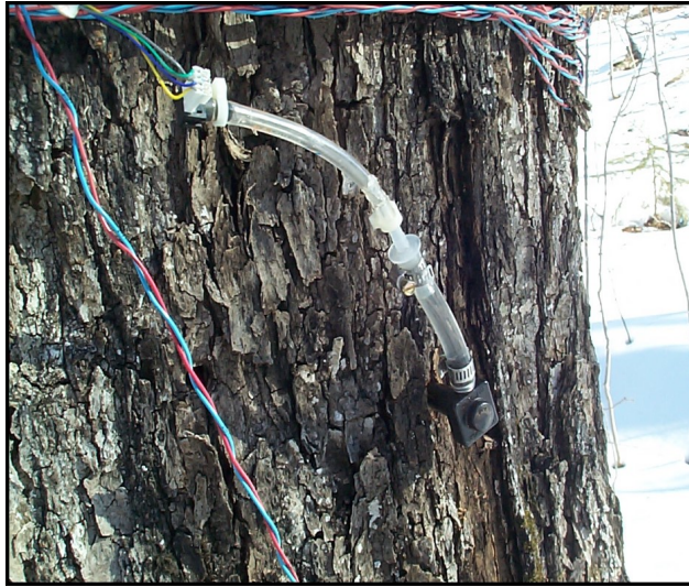
Figure 1: Photograph of a taphole containing a black nylon spout that is connected by plastic tubing to an Omega PX-26-030GV pressure sensor. Additional wires leading to thermocouples are also shown.
