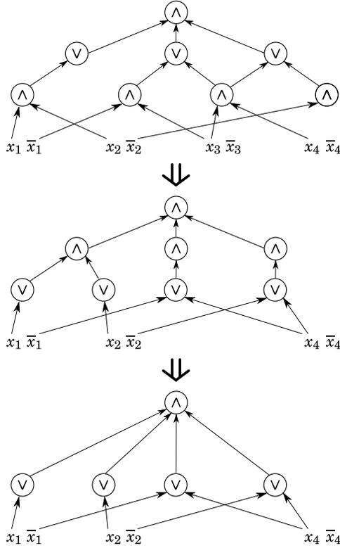
**Figure 4.2.** At top is the initial circuit. Under the restriction fixing  $x_3 = \text{True}$ , all three DNFs at layer 2 may be replaced by CNFs of width at most 2. Finally, the nodes at layers 2 and 3 may be compressed.
