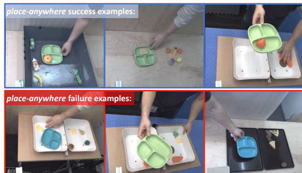
Fig. 4: Video frames for the place-anywhere task. Success and failure videos are iteratively captured in pairs to mitigate correlations with spurious workspace features such as hands of the user, backgrounds, bins, and distractor objects.
