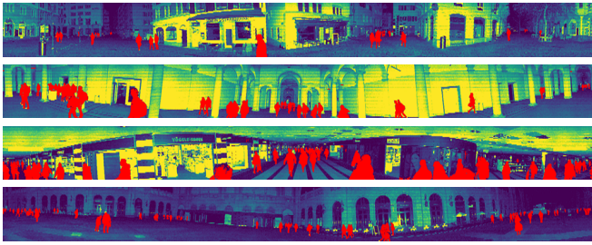
Fig. 5. Occupancy grid based detection examples shown on the intensity image generated from the point clouds. Detected dynamic objects are colored in red. Top to Bottom: Niederdorf, Hauptgebäude, Shopville, Station.
