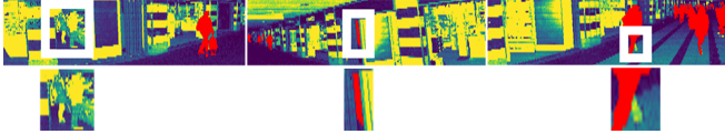
Fig. 6. Examples of erroneous annotations in the dataset: Left: Missed detection from under-segmentation: Humans are close to a shelf and end up in a cluster with it. Middle: False positive resulting from reflective surfaces. Right: The object is detected, but the lower leg is missing.
