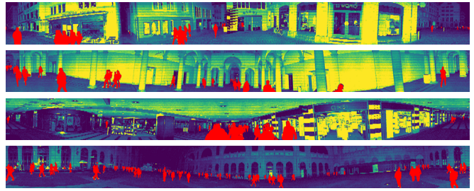
Fig. 7. 3D-MiniNet prediction examples at the four different locations. For each location, the training was performed on the automatically labeled data of the 3 remaining locations.
