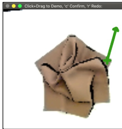
Fig. 8: The user interface for human interventions. The current observation of the fabric state from the robot’s perspective is displayed, with an overlaid green arrow indicating the action the human has just specified.
