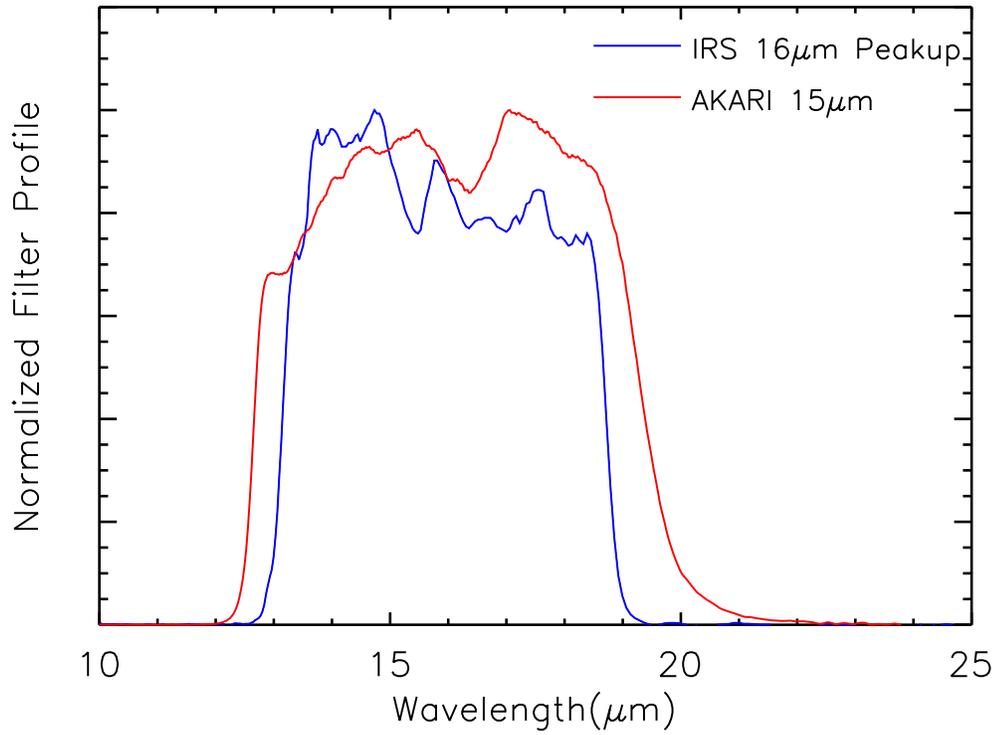
**Figure 1.** Normalized filter transmission profiles. Red line shows the *Akari*/IRC 15  $\mu\text{m}$  profile, and blue line shows the *Spitzer*/IRS 16  $\mu\text{m}$  peakup imager profile. The *Akari* 15  $\mu\text{m}$  filter profile in general overlaps with but is slightly wider than the IRS 16  $\mu\text{m}$  profile.
