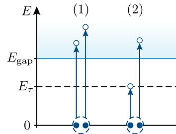
FIG. 2. Two types of energy absorption processes that may contribute to  $\text{Re} Y(\omega)$  at  $T = 0$ . In processes of type (1) a drive photon breaks a Cooper pair into two above-the-gap quasiparticles [ $E > E_{\text{gap}}$ ]. In processes of type (2) a Cooper pair breaks into one quasiparticle at the discrete in-gap state,  $E = E_\tau$ , and one quasiparticle above the continuum's edge,  $E > E_{\text{gap}}$ .
