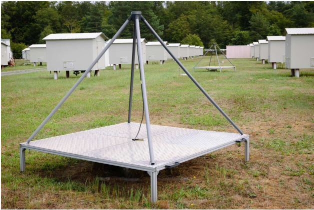
Fig. 1 Photo of an inverted v-shape dipole antenna of the LOPES-30 setup in the KASCADE particle-detector array.
