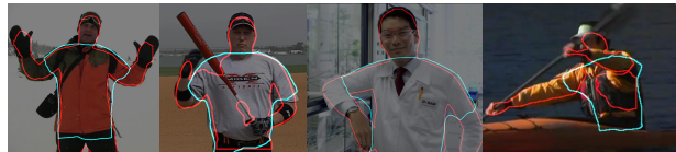
Figure 13. The qualitative silhouette comparison between the detected densepose mask (red) and the boundary of 3D clothes retargeted by ours (blue). Notice that densepose mainly detects the inside of the body, while CRNet captures semantically more meaningful clothing boundaries.
