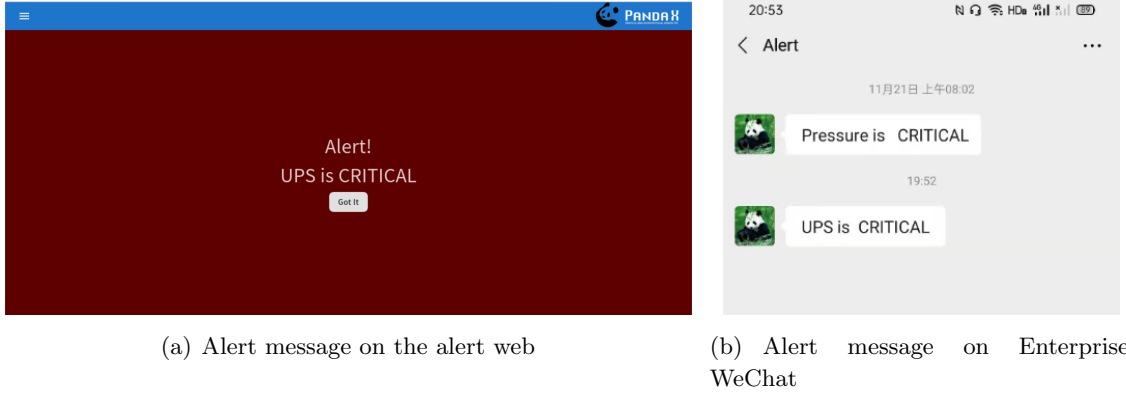
Fig. 11. An alert message was generated by the accident of input power cut of the UPS. The message is displayed on the web (a) and delivered to users by the Enterprise WeChat (b).
