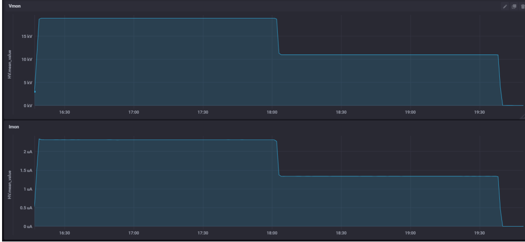
Fig. 6. Example of the voltage (top) and current (bottom) from the Matsusada AU HV power supplies during a data taking run, collected by the P-SCS.
