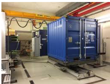
Figure 3.15: Movable support structure for concept evaluation. Its movement degrees of freedom allow 3D \gamma -ray beam scanning for “real-world” scenarios. This figure is adapted from a paper by kolokytha et al. [136] of the CEA Saclay in France.
