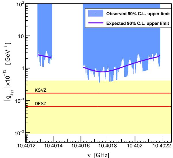
FIG. 5. The 90% single-sided C.L. upper limit for the axion coupling constant  $g_{a\gamma\gamma}$ . Each point corresponds to a test axion mass in the analysis window. The solid curve represents the expected limit in the case of no signal. The yellow region indicates the QCD axion model band. We assume  $\rho_a \sim 0.45$  GeV/cm $^3$ .
