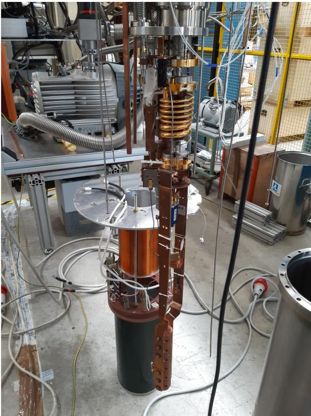
FIG. 1. View of the QUAX- $a\gamma$  dilution refrigerator insert, instrumented with the resonant cavity (at the bottom) and amplification chain. In the background, the 8.1 T magnet with its countercoil is visible.
