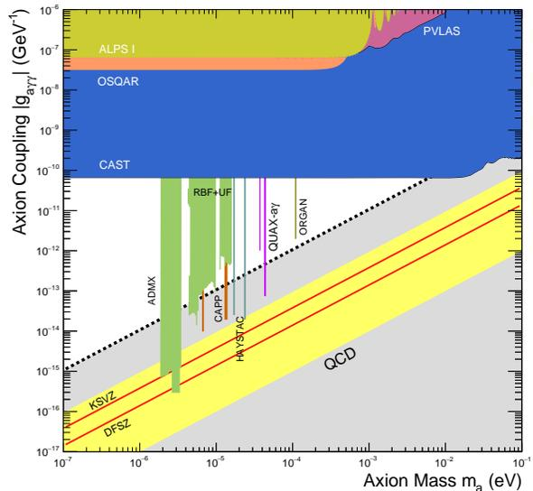
FIG. 6. Aggregate plot of the limits on  $g_{a\gamma\gamma}$  obtained from the main axion search experiments. The two limits obtained by the QUAX Collaboration are highlighted in purple. The gray area identifies the region where axions could be found, with the yellow band and the two solid red lines identifying the coupling predicted by the KSVZ and DFSZ models and its uncertainty.
