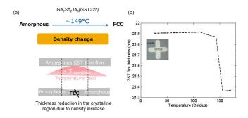
FIG. 5. Calibration. (a) Cartoon to show the phase transition in  $Ge_2Sb_2Te_5$ . (b) Inset: Optical micrograph of the calibration sample. Main: Thickness (measured using AFM, with vertical resolution of 0.05 nm) of the calibration sample as a function of oven temperature. The glass transition temperature  $T_g$  is 149°C.
