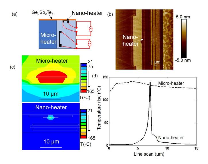
FIG. 1. Heat sources inside the head of the hard disk drive. (a) Cross-sectional cartoon of the head structure showing the embedded heat sources: the nano-heater and the micro-heater. (b) AFM image of the device: the micro-heater is embedded and cannot be seen from the surface, while the nano-heater is located at the center. The dimension of the nano-heater is 1  $\mu$ m × 20 nm. (c), (d) Simulation: Temperature map of the nano-heater and the micro-heater with similar peak surface temperature.
