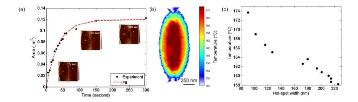
FIG. 3. Time response of  $Ge_2Sb_2Te_5$  at a constant nano-heater power of 0.68 mW. (a) The transition area of  $Ge_2Sb_2Te_5$  phase change with the the accumulated heating time. (b) Shows the temperature map of the nano-heater. (c) Shows the temperature as a function of the hotspot width across the nanoheater.
